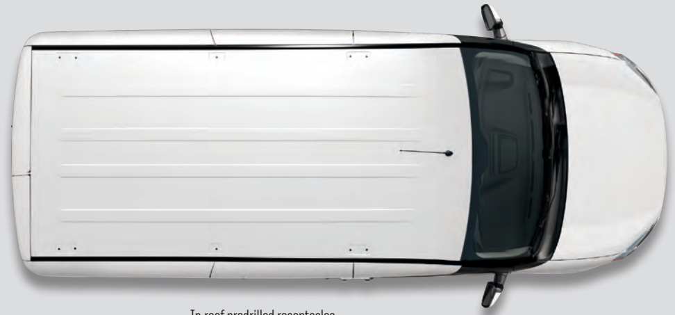
In-roof predrilled receptacles
